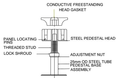
electrical conductive gasket is placed on top of the pedestal head to eliminate rattles and improve sound insulation. Each pedestal head has an adjustment nut shroud to insure pedestal height is maintained.
